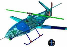
HADA is a hybrid vehicle that takes off as a helicopter and flies as an airplane. The UAV retract the rotor blades and spread the wings when the velocity is high enough. The engineering around the mission specification is critical, given the impact on the aircraft design and final performance. The strategy to run the transition between both modes of operation, as well as the propulsion requirements to carry it out, is part of the current research.
