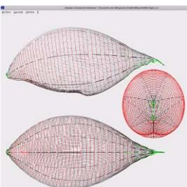
Structural analysis of inflatable structures and their behaviour when acting as buoyancy or lifting shapes. The model can reconstruct the final geometry from initial flat patches, inflation pressure and external airflow.
