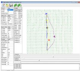
Given the dependency of aircraft performance from the meteorological conditions, a research line exploits the benefits of having a better knowledge of atmospheric conditions in real time. Thus, analytical methods (in contrast to other extended approximate solutions) are used to find best trajectories for several figures of merit, including weather forecast modifications and the occurrence of path constraints.
