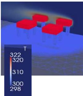
Heat transfer analysis is just one of the capabilities of the CFD codes with a broad range of applications. As a remarkable effort, some simulations have been conducted in order to predict performance features of the wind sensor of the REMS station, onboard the Curiosity rover on Mars. It is able to measure Martian wind speed and direction as a function of the heat evacuated from small heated dices.
