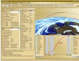
The ascent optimal trajectory for small launchers can be calculated for injection at maximum orbital height with autonomous rapid corrections in real time. The angle of thrust vector -the single control- can be solved together with some system design parameters by applying an indirect optimization method iterated over the parameter space. Feasibility, accuracy and convergence of the method are part of the research, as well as necessary throughput.
