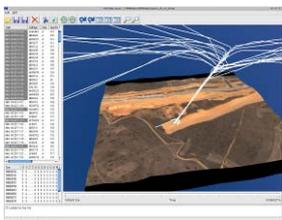
Some of the phases of an aircraft mission are easily predictable. When aircraft trajectory is known, differences between expected and real path can be due to meteorological conditions. Dedicated filters can be used to deduce the wind field from large dataset of real trajectories. The method is completed with meteorological models to obtain better initial estimations and with real time measurements to improve accuracy.
