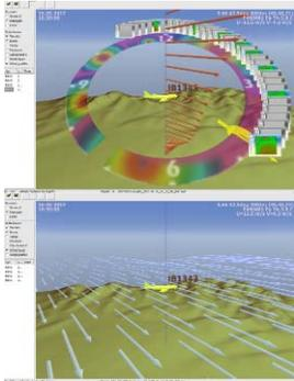
Customised 4D weather forecast models to deliver digital meteorological data with sufficient resolution and accuracy for autonomous air traffic management. This is normally based on multi-weather-model multi-analysis ensemble prediction systems with real time assimilation of external data. Currently, the research focuses on:
