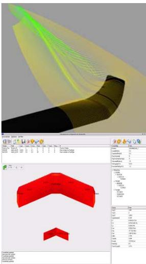
Low speed aerodynamics applies to objects moving through fluids of constant density, typically when object speed is below 0.3 Mach. It is a relatively simple flow that involves a lot of industrial design problems. Numerical modelling is a very useful tool as it helps to reduce wind tunnel tests during the design process, which implies lower development costs.
